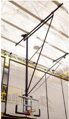
■ TBS-26-B Basketball Backstop features bolt-together main frame for all heights. Specify left or right side fold. It comes with a single brace located back or front as required. Backstops are custom designed so the lateral sway brace intersects the main mast at approximately 54" (1.37 m) above the goal and 18" (46 cm) above the backboard; to ensure maximum rigidity.
